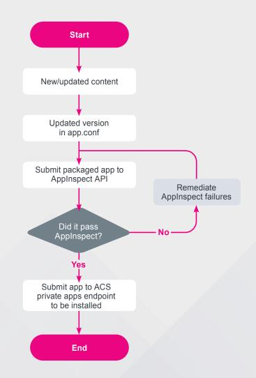
When automating AppInspect into your workflows, we recommend running AppInspect against any private apps that have changed in that branch before the merge request that will attempt to deploy the changes is run. This will ensure that AppInspect issues are caught early and will minimize any potential issues just before deployment, even though it is possible that you might still push the apps through AppInspect again during the deployment.
