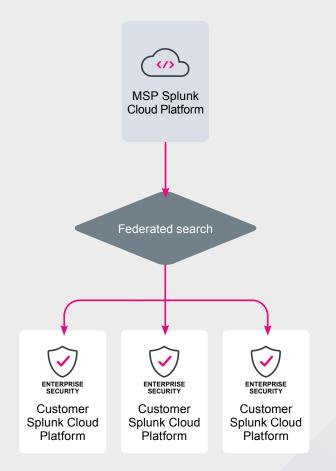
This will mean that you will be able to aggregate notables into a dashboard on the MSP environment. Analysts, however, will need to navigate to the customer's Enterprise Security instance to perform investigations.
